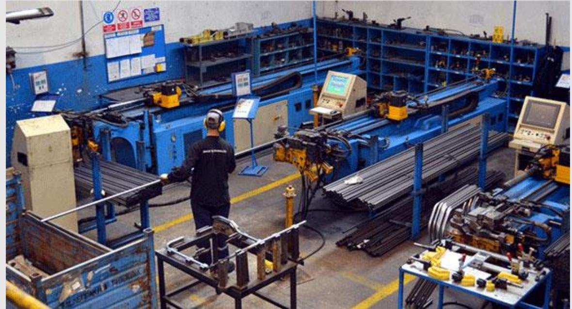
*We are capable to bend and shape pipes within the range of max 4600 mm stroke lenght ,with max diameter 38 mm and max 190 degree.*
